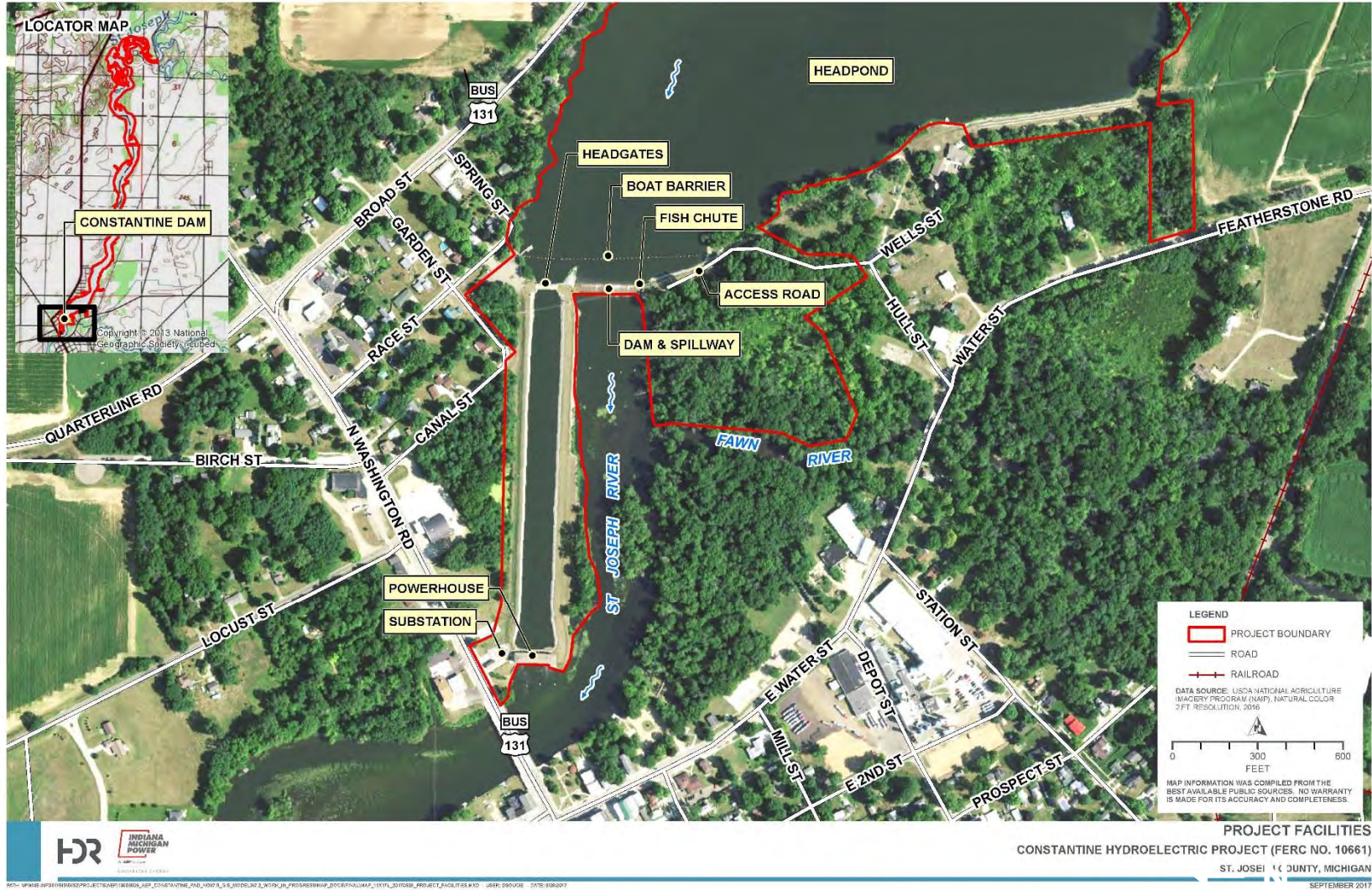
Figure 4.2-2 Aerial View of Project Facilities
